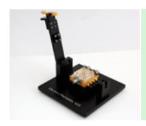
The FRFS-A0800 is a high performance RF/Microwave production type fixture for testing RF Micro Devices amplifier P/N RF2186. This fixture is constructed to provide repeatable measurements in a production environment. The FRFS-A0800 test fixture feature fast load/unload clamshell type cover.
