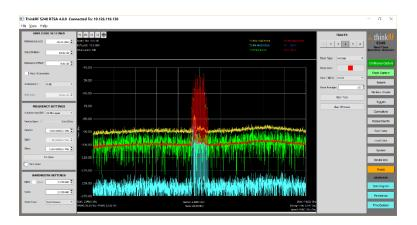
By utilizing the power of the R5500, the S240 application has all the standard features you expect from a traditional lab spectrum analyzer as well as powerful features such as real-time triggering.
