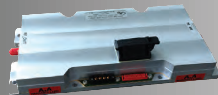
Module -0 Conduction through baseplate
