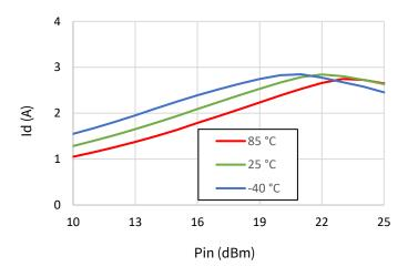
Figure 26: Ig v. Pin v. Temperature
