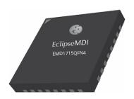
Eclipse Microdevices EMD1715 is a GaAs MMIC PHEMPT distributed general purpose low noise amplifier. This LNA has a small signal gain of 14 dB with noise figure less than 2.3 dB at 6 GHz. This device is ideal for applications that require a typical P1dB output power of +20dBm up to 12 GHz, while requiring only 103mA from a + 5 Volt supply.
