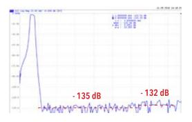
Typical dynamic range of 130 dB is achieved from 300 kHz through the top of the frequency range (at 10 Hz IF bandwidth). Seen here is the maximum dynamic range achieved when using IFBW 1 Hz and an output power level of 5 dBm.
