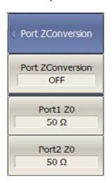
This function converts the S-parameters measured at a  $50\Omega$  port into values which would be seen if measured at a test port with arbitrary impedance.
