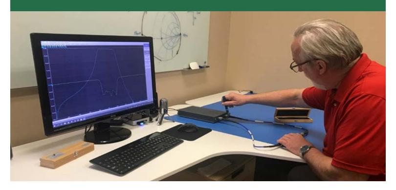
M Series VNAs deliver metrology-grade performance in a more economical package that excludes a number of advanced features. These Vector Network Analyzers are small, can be powered by battery, and are ideal for use in laboratory and production testing in a variety of applications including filter tuning, antenna test and characterization, amplifier testing, etc.
