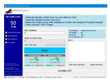
On-screen instructions guide the operator through each step of the work order testing process. If a device fails a test, the operator has the option to re-test. Test statistics are displayed and recorded. While testing a work order, VNA screenshots can be saved or printed. The operator closes the work order once all devices have been tested.
