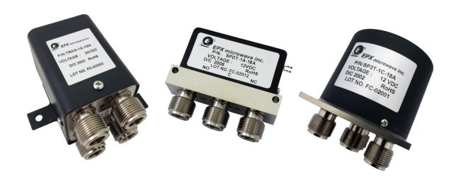
EPX Microwave announces a new series of coaxial switches, extending the usual N connector frequency range of DC~12.4 GHz to DC~18 GHz. Each model is available with the option of built-in internal terminations. The series includes single pole double throw, transfer and single pole multi-throw models up to 12 ports.
